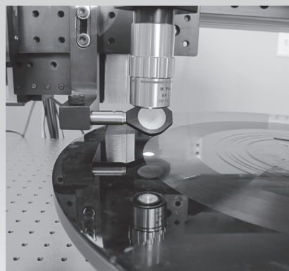
IRENE's 2D camera images the grooves on a lacquer disc.
